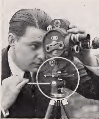
New focusing alignment gauge in use
